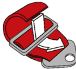
STEP 4: Fold back strap again and insert through bottom portion of buckle.
